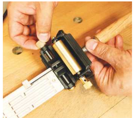
▲ ... and then clamped securely by winding in the brass knob until it nips
